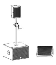
The G Sub 1501 dp++ features integrated digital amplifier electronics with a DSP controller. Various factory-configured presets and volume settings can be selected.
