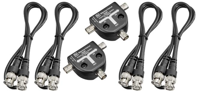
The PASP is a passive antenna splitter kit containing necessary items when splitting and sharing two incoming antenna signals between the diversity antenna jacks of two receivers. An ideal companion kit to the RMK2 dual rack kit, the PASP takes the signals collected by the front-mounted antennas on the RMK2's CXU2 jacks, and distributes them to the diversity antenna input jacks on two receivers. Will adapt any other sources of incoming cable-bound RF signals via BNC from remote antennas.
