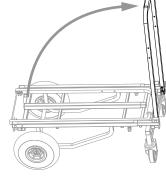
To extend the length of the loading surface, loosen the two hand screws at the bottom of the frame.
