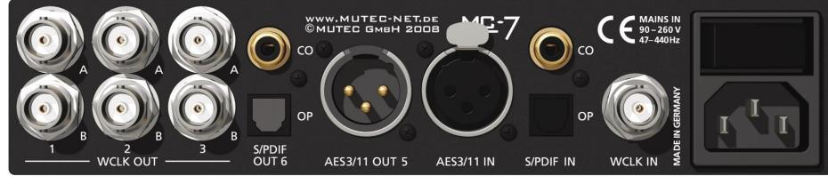
**The MC-7 is a flexible, high performance 8 channel Word Clock distribution amplifier and audio clock converter**
