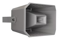
The MPLT32-G is two-way long throw horn 100 volt high quality music projector. It has 32 watts rated power handling RMS at 100 volt and has transformer taps at 32 - 16 - 8 - 4 watts. Its long throw output performance brings quality sound over long distances and in wide areas with both music and speech. The two-way characteristic makes your music still sound natural where the horn shape housing makes sure you cover a big distance.
