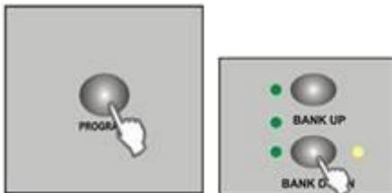
Power off the unit. Press and hold down the Program and Bank Down buttons at a time while switch on. All scenes and chases would be cleared.
