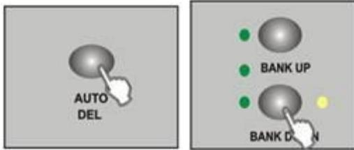
Power off the unit. Press and hold the Auto/Del and Bank Down buttons at the same time while switch on. All chases will be deleted.
