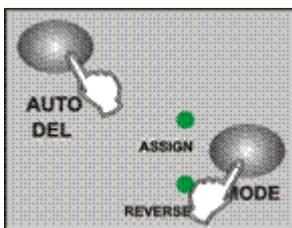
Power off the unit. Press the Mode and Auto/Del buttons at a time while switch on. All LEDs should flash briefly, indicating all assigned or reversed DMX channel are cleared.
