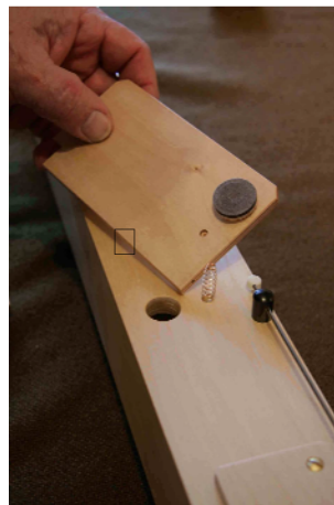
Countersink for the spring
