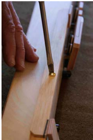
Filing the cork on the key levers
