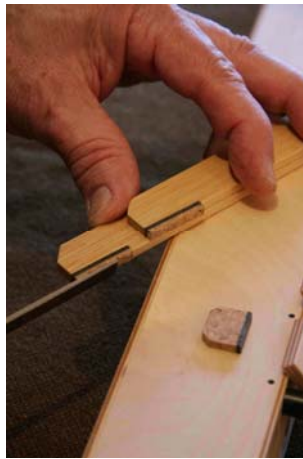
Filing the cork on the key levers
