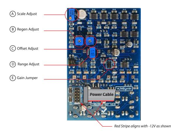
A Scale Adjust: Sets the 1V/Oct voltage scaling. To adjust, first remove all inputs, then turn Emphasis
