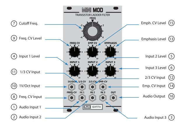
1 Audio Input 1: Audio Input 1 forms part of a 3 input audio mixer which is attached to the front end of the filter. This Input is mixed with Input 2 and Input 3 at a level set by Audio 1 Level control (4). Typically the output from a VCO would be connected to this Input, but any AC signal with a level of up to +/- 5 Volts is acceptable.
