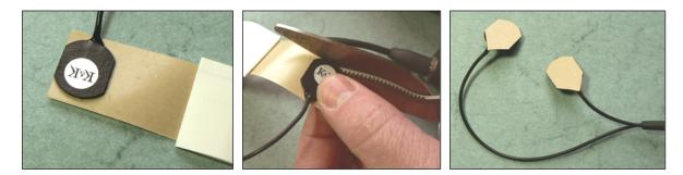
We recommend applying two layers of the double stick tape. After the first layer is applied as shown, peel off the brown protective tape. Repeat the procedure. This helps to reduce the sensitivity towards unwanted mechanical transmissions and guarantees the most secure adhesion.
