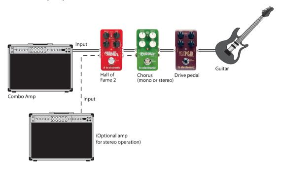
When using the HALL OF FAME 2 before the amp's input, it is generally best to place it after your other pedals. If any stereo effects are used before the reverb pedal, you can preserve this stereo signal by connecting to both of the HOF's inputs and sending the output jacks to different amps or to a stereo input on a mixer.
