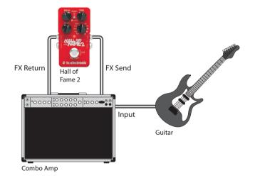
The HALL OF FAME 2 has a very wide gain range, and can easily be used with guitar or loop-level signals. Simply connect the amp's Send jack to the HOF input, and connect the output to the amp's Return jack.
