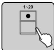
3. Press the number button [1 – 20] where the desired chase is stored. The LED of the [BANK] button lights up and the display shows the number and the chase parameters for BANK, SCENE, STEP, FADE and WAIT. Additionally, the LEDs of those number buttons [1 – 20] are flashing, where scenes have already been assigned to in the respectively displayed bank.
