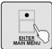
4. ➤ Press the [ENTER / MAIN MENU] button to confirm, all LEDs blink three times. Then, the device will quit this submenu.
