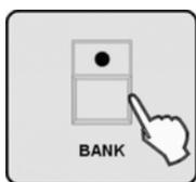
1. ➤ Press the [BANK] button and turn jog wheel # 1 to select the desired bank 1 – 60.
