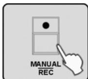
**5.** Press the *[MANUAL/REC]* button - now the LEDs of the buttons CUE, OVERRIDE, CENTER, FIXTURE GROUP, PRESET, CHASE, BANK and BLACK OUT are flashing.
