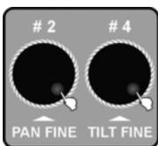
**3.** Turn jog wheels # 2 and # 4 to enter the name of the fixture. Rotate jog wheel # 2 to change the cursor position. Turn Jog wheel # 4 to change the character. You can choose from 26 letters and 10 numbers as well as the special character '—'. The max. length of the device name is 16 characters.
