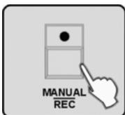
6. ➤ Press the MANUAL/REC button to initiate the saving. The LEDs of the buttons CUE, OVERRIDE, CENTER, FIXTURE GROUP, PRESET, CHASE, BANK and BLACKOUT are flashing.
