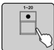
2. ➤ Press the number button [1 – 20] to select the desired chase. You can also select multiple chases. Their numbers will be indicated in the display. The number of the currently active Chase is flashing then. To activate the respectively next Chase, press the number button [1 – 20] of the currently active Chase in order to deactivate it.
