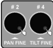
7. Turn jog wheel # 2 to select the field for the desired channel. Turn jog wheel # 4 to change the function assignment for the current channel (e.g., PAN, TILT, DIM, etc.).
