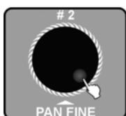
3. ➤ Rotate jog wheel # 2 to select '[inside time]' or '[outside time]'. If '[inside time]' is selected, the chase run is controlled by the time values used during programming the individual scenes. If '[outside time]' is selected, the timing can be freely adjusted during the chase run.
