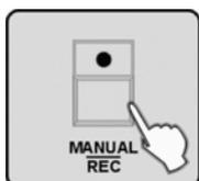
6. ➤ Press the [MANUAL/REC] button - now the LEDs of the buttons CUE, OVERRIDE, CENTER, FIXTURE GROUP, PRESET, CHASE, BANK and BLACK OUT are flashing.
