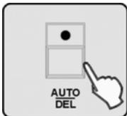
3. ➤ Hold down the [AUTO/DEL] button while pressing the number button [1 – 20] of the Chase to be deleted. All LEDs flash three times and thus indicate the successful deletion of a Chase.
