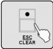
Press the *[ESC / CLEAR]* button to return to the previous menu level. Press repeatedly to finally leave the menu.
