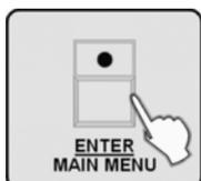
6. ➤ Press the [ENTER / MAIN MENU] button to confirm. All LEDs will flash three times, thus indicating the success of the procedure.
