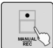
4. ➤ Press the [MANUAL/REC] button - now the LEDs of the buttons CUE, OVERRIDE, CENTER, FIXTURE GROUP, PRESET, CHASE, BANK and BLACK OUT are flashing.
