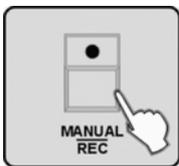
**3.** Press the *[MANUAL/REC]* button - now the LEDs of the buttons CUE, OVERRIDE, CENTER, FIXTURE GROUP, PRESET, CHASE, BANK and BLACK OUT are flashing.
