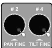
**5.** Turn jog wheel # 2 to select the field for the desired channel. Turn jog wheel # 4 to change the function assignment for the current channel (e.g., PAN, TILT, DIM, etc.). The attributes 'A' (amber) and 'W' (white) are supported.
