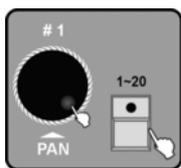
5. ▶ Rotate jog wheel # 1 to select the bank that contains the scene that you want to insert. Press the number button [1 – 20] of the scene to be added to the chase in the current step.
