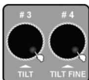
**8.** Turn jog wheel # 3 to adjust the FADE TIME for the current Chase. Turn jog wheel # 4 to adjust the WAIT TIME for the current Chase. If you don't adjust these settings, the device will take over the most recently used values for FADE TIME and WAIT TIME.
