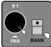
**5.** Press the *[BANK]* button. Then rotate jog wheel # 1 to select the bank to which you want to copy the scene.
