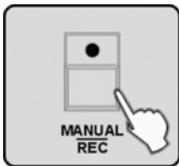
**8.** Press the *[MANUAL/REC]* button - now the LEDs of the buttons CUE, OVERRIDE, CENTER, FIXTURE GROUP, PRESET, CHASE, BANK and BLACK OUT are flashing.
