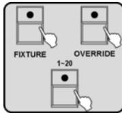
1. ▶ While CUE, CHASE or BANK scenes are running, press the *[OVERRIDE]* button. Then press the *[FIXTURE]* button and subsequently use the number button *[1 – 20]* to select the device whose effect you want to change manually. Move the faders or turn the jog wheels 1 – 4 to modify the effect.
