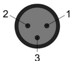
Two female 3-pin XLR sockets are used for the DMX output. The following figure and the table show the sockets' pin assignment.
