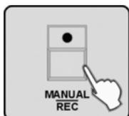
7. ▶ Press the [MANUAL/REC] button. All LEDs flash three times and thus indicate the successful replacement of a scene.
