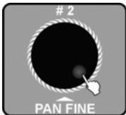
3. ➤ Turn jog wheel # 2 to switch from the default setting '[stand by]' to '[pan/tilt center]' or '[black out scene]'.
