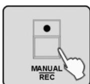
5. ➤ Press the [MANUAL/REC] button. All LEDs flash three times and thus indicate the successful editing of a Cue. The Cue run is stopped then.
