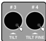
6. ▶ Turn jog wheels # 3 & # 4 to adjust the FADE and WAIT TIME for the current scene. If you don't adjust these settings, the device will take over the most recently used values for FADE TIME and WAIT TIME.
