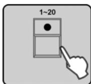
6. ➤ Press the number button [1 – 20] to select a memory slot for the Center. All LEDs flash three times and thus indicate the successful saving of a Center position. All set DMX values that are not related to PAN & TILT are not saved.
