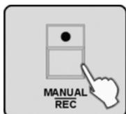
7. Press the [MANUAL/REC] button, all LEDs blink three times and all scenes of the selected bank have now been added to the current Chase.
