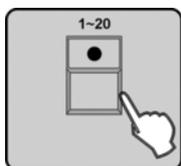
5. ➤ Press the number button [1 – 20] to select the number for the fixture group. All LEDs flash three times to confirm.
