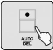
5. ➤ Press the [AUTO/DEL] button. All LEDs flash three times and thus indicate the successful deletion of a scene.
