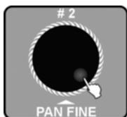
3. ➤ Turn jog wheel # 2 to switch to the previous or next programmed step within the active Chase.
