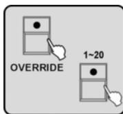
1. ▶ While CUE, CHASE or BANK scenes are running, press the *[OVERRIDE]* button. Now the LED of this button flashes along with the LEDs of those number buttons *[1 – 20]* where Overrides have already been programmed. Press the number button *[1 – 20]* to activate the desired Override. The LED of this button lights up then.
