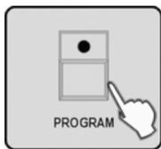
Enter the programming mode by holding down the *[PROGRAM]* button for 2 seconds. The LED of the *[PROGRAM]* button flashes when the programming mode is activated.
