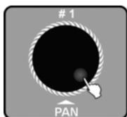
6. ➤ Rotate the jog wheel # 1 to select the number of the preset group 1 – 20, to which the current settings for colour and gobo wheel are to be saved.
