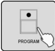
1. ➤ Enter the programming mode by holding down the *[PROGRAM]* button for 2 seconds. The LED of the *[PROGRAM]* button flashes when the programming mode is activated.
