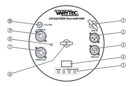
1 Safety cable eyelet. 2 [DMX IN] DMX input, designed as 3-pin XLR chassis-mounted plug 3 [DMX OUT] DMX output, designed as 3-pin XLR chassis-mounted coupling 4 Display 5 Operating buttons [ENTER] Confirms a selected value. [DOWN] Decreases the displayed value by one. [UP] Increases the displayed value by one.
