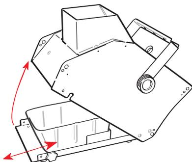
Once the screws are removed, the lid of the housing can be carefully swung upwards, as shown above and the fluid tank can be removed for refilling. Take care not to spill any of the bubble fluid inside the unit. The fluid tank is designed to fit only one way around. Make sure you insert it correctly, as shown above, with the lower edge facing into the machine.
