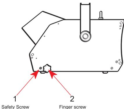
Remove the two safety screws on both sides of the device with the required screwdriver. (see drawing, 1). Once these are removed, the finger screws can be undone by hand (see drawing, 2).
