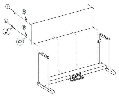
Slide in the rear cover before the small angle pieces and attach the rear cover with two Phillips screws M4  $\times$  12 and washer. Now affix the rear cover with four Phillips screws ST3 9  $\times$  16 and washer to the pedal box.
