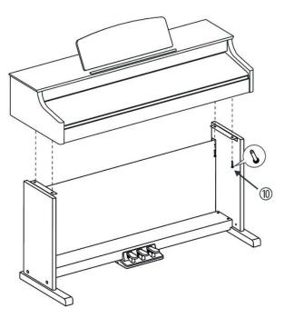
Place the digital piano case on the frame and secure it with four Phillips screws M6  $\times$  16.
