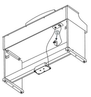
Fasten the cables to the stand. Insert the DIN plug of the pedal cable into the provided socket on the bottom side of the digital piano. Move the digital piano to its designated location.
