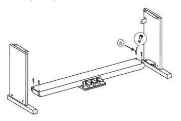
**3.** Screw the levelling bolt on the bottom of the pedal box completely in.
