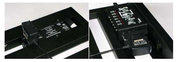
To secure the connection you can use a rubber band or a cable tie to fix the adapter to the bracket as shown below.
