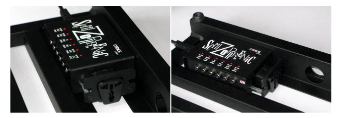
When a link type power supply is mounted underneath the Pedaltrain board as described earlier in this document, the adapter allows powering of two different devices like ex. a plug-in adapter – one plugged in from the top and one placed underneath the board as shown on following two pictures.
