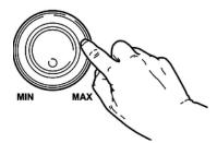
Turn the volume knob counter-clockwise to minimum before connecting the digital piano to the power supply or to other devices. This is to protect the speakers from damage.
