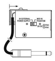
To connect the cables remove the fixing cover. After connecting them put it back, press down and tight up (see the picture below).
