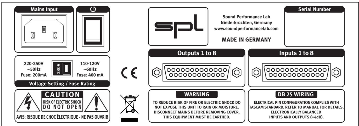
The electrical pin configuration of the balanced DB 25 input and output sockets comply with the TASCAM standard (see graphic below). The nominal input level is +4 dB, other levels are transmitted 1:1.
