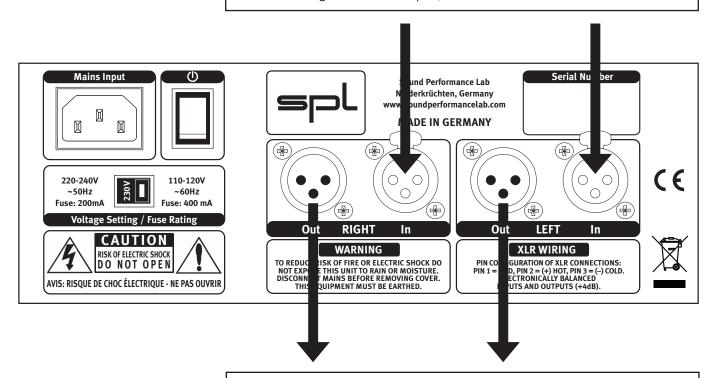
**Balanced right and left XLR Outputs** to provide for connections to power amps or active speakers.
