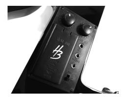
Replace the inserted batteries if necessary (weak output signal) or at regular intervals. Open the battery compartment cover on the back of the instrument.
