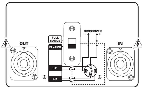
Fig. 1.1: Connector panel on multi-way systems (except B1020)
