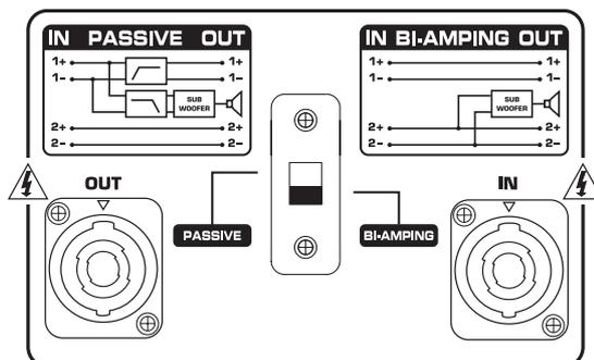
Fig. 1.3: Connector panel on subwoofers
