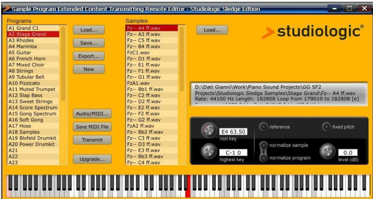
SAMPLES can be transmitted to the internal 60 megabyte of internal flash memory (already installed in every SLEDGE) by the dedicated program SLEDGE SPECTRE, that allows to send samples to Sledge in various formats, edit their basic parameters (tune, keyboard range for each sample etc) and play the SAMPLES on your computer and make a full musical test before sending them to the instrument.
