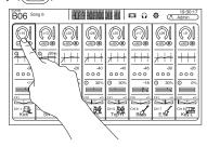
You can switch between the FADER section and the CH STRIP section by pressing the home key while the OVERVIEW screen is displayed.
